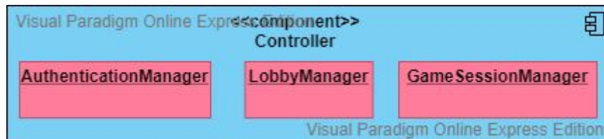
Figure 10: Controller component and its classes
